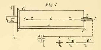
2. Apparatus.—This consists of a cylinder of glass C, F, about 45 cm. long, 13.4 cm. internal diameter, closed at one end F and provided with a brass cap C, with exhaust E and influx attachments I, in the usual way. There is a layer of water w at the bottom. The glass must be scrupulously clean within; and this is best secured by scouring with a probang of soft rubber under water, until the water adheres as an even film on shaking. The fog chamber is put to earth, as at e.
